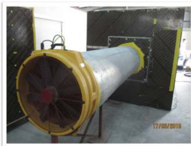
Rear end of test chamber with fan
