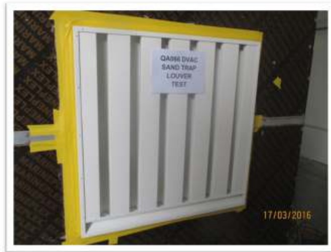
Pressure Drop Test Set-up (Front End with mounted sample)
